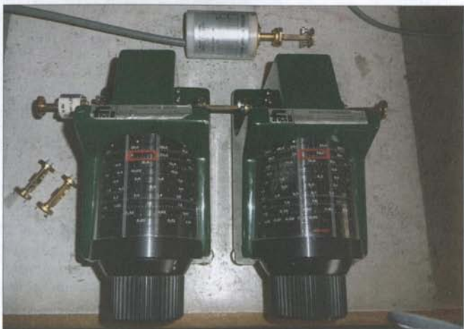
Fig. 4: Flann Rotary Attenuator 2711 with up to 70 dB attenuation.
