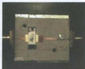
A 50 W 9cm Test Amplifier by G3WDG using the GaN-Transistor T1G4005528-FS from TriQuint
