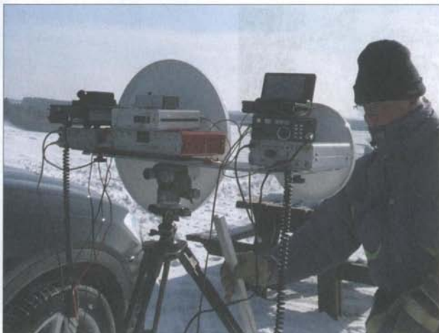
Fig. 1: Setup for 76 and 122 GHz and GPS RX at DL2AM/P in JN47WA in February 2012
