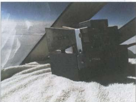
N0SP/AM 10 GHz 30 mW beacon transmitter in the front window of a private jet aircraft at 15000 Meters
